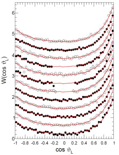
Integral angular distribution of PFN relative to the fission axis
