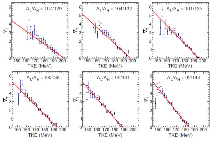
Slope gives directly the change in TXE per emitted neutron
