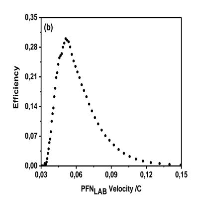
The efficiency of ND was evaluated by comparison of TOF distribution with Maxwellian distribution with the temperature parameter 1,31 MeV,  $\bar{\nu}=2.44$  and the flight path 0,65 m, Fig. (a). The conversion from TOF to PFN velocity distribution is plotted in Fig. (b).
