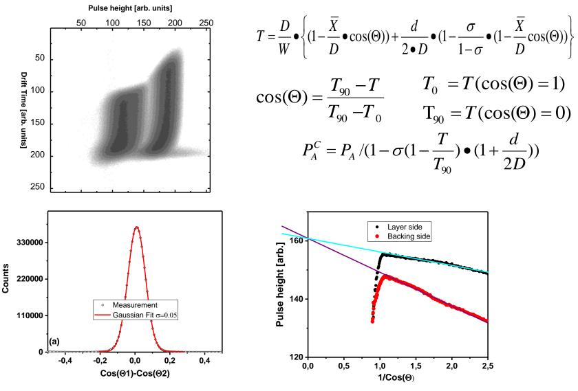
Cosine values determined according the algorithm described in previous slide are plotted in two dimensional plot of cosines measured in both halves of TBIC to demonstrate the quality of the algorithm.
