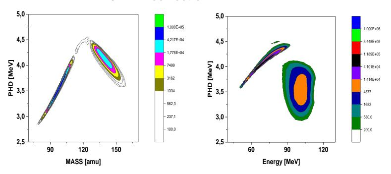
PHD was measured for P-10 working gas by C. Budtz-Jorgensen and tabulated. For FF pulse height corrections in the Ref.: F.-J. Hambsch, J. van Aarle, and R. Vogt, Nucl. Instrum. and Meth. A361, 257 (1995) the following parameteresation of the tabulated data was suggested which is more convenient for data analysis:
