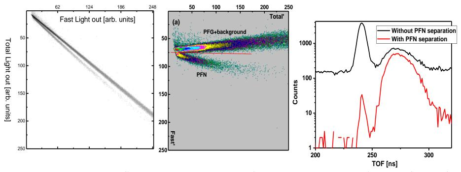
The two window algorithm (fast and total light output component) was implemented and resulted function *ND(Fast,Total)* was plotted on the upper and middle figs. demonstrates the function *ND(Fast,Total)* in rotated according to equation
