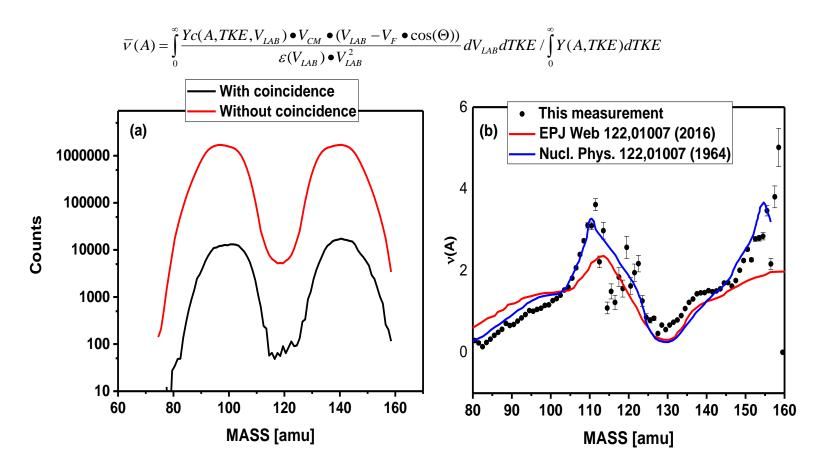
FF mass and Energy values were corrected in iterative mass&tTKE evaluation procedure, described in F.-J. Hambsch, J. van Aarle, and R. Vogt, Nucl. Instrum. and Meth. A361, 257 (1995), but corrected for FF recoil according to A. Gavron, Nucl. Instrum. and Meth., 115 (1974) 99
