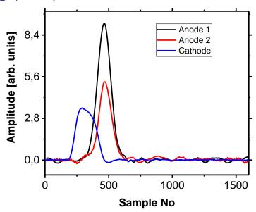
In our approach we have oversampled FF signals. The oversampling we used to increase the effective number of bits (ENOB) improving the signal representation. In practice the increase of ENOB realized automatically when signal passed through second order low pass filter:
