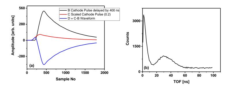
The realization of the algorithm demonstrated in Fig. (a) as it was applied to the cathode waveform. The copy of the original signal is delayed by approximately 0.4 of the cathode signal rise time (~1000 ns) and summed with scaled (0.2) and the inverted original signal. The "T-zero" time is assigned to the crossing point of resulting signal with time axis.
