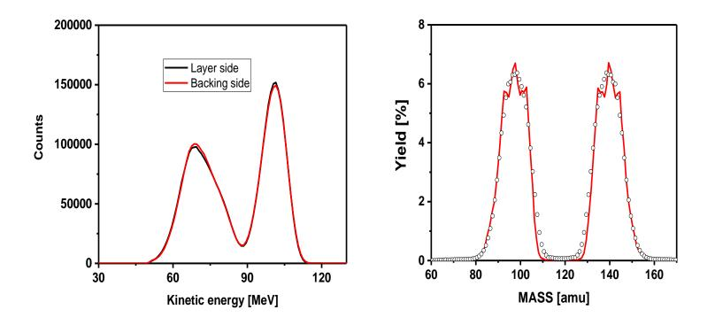
The left distribution demonstrates accuracy of implemented corrections in FFs kinetic energies. In the right plot the comparison of measured mass distribution with the literature (C. Wagemans, The Nuclear Fission Process, CRC Press, Boca Raton, FL, 1991, p. 300) is presented.
