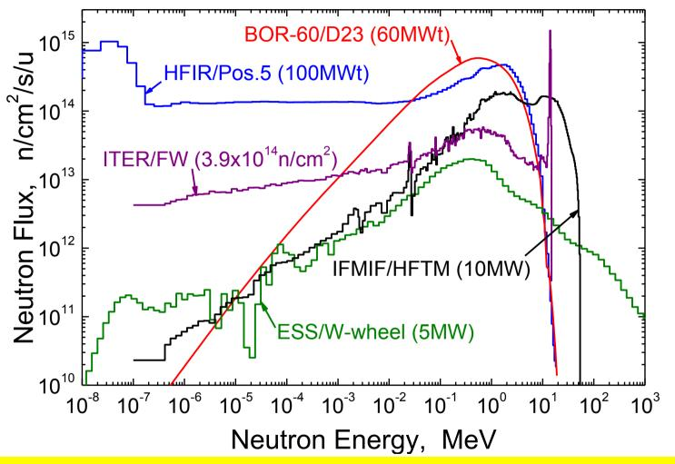
For representative calculation of SPA we selected: HFIR/C5 (Fission), ITER/FW (Fusion) & IFMIF/HFTM (Spallation)
